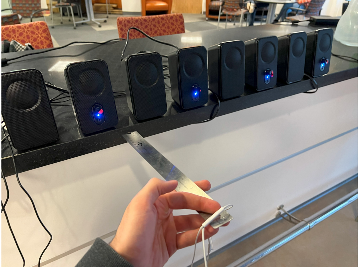
Figure 11. An image showing how I held the microphone and ruler to collect the data. I needed a hand to take the picture, so in reality, I was dangling the microphone just a little bit above the end of the ruler.
