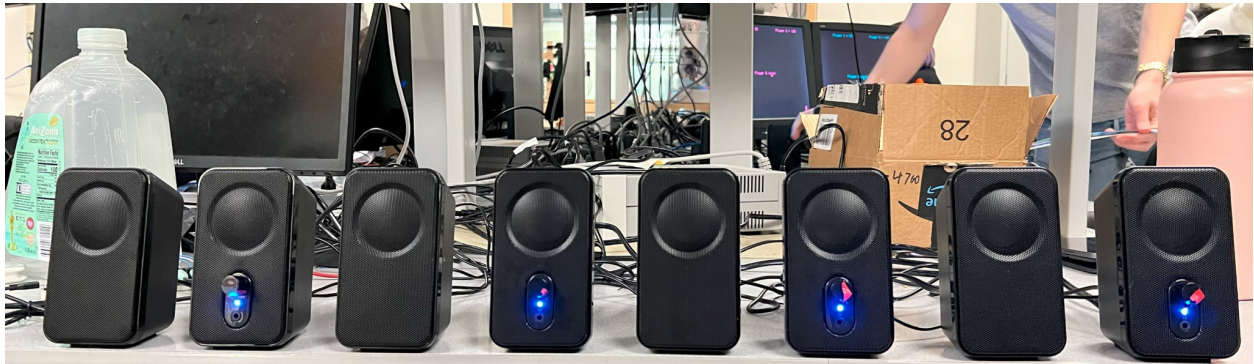
Figure 9. An image, showing off all eight speakers of the speaker array. The red tape on the right speakers of each pair of speakers was used to keep all the volumes of the speaker pairs all the same.
