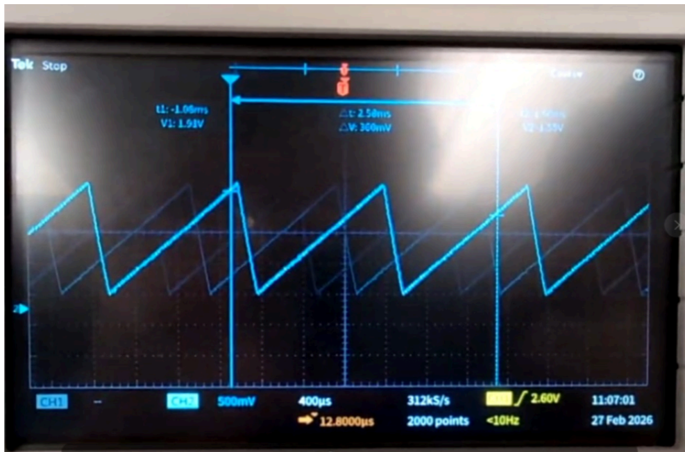
Figure 6. Triangle audio display using MCP4822
