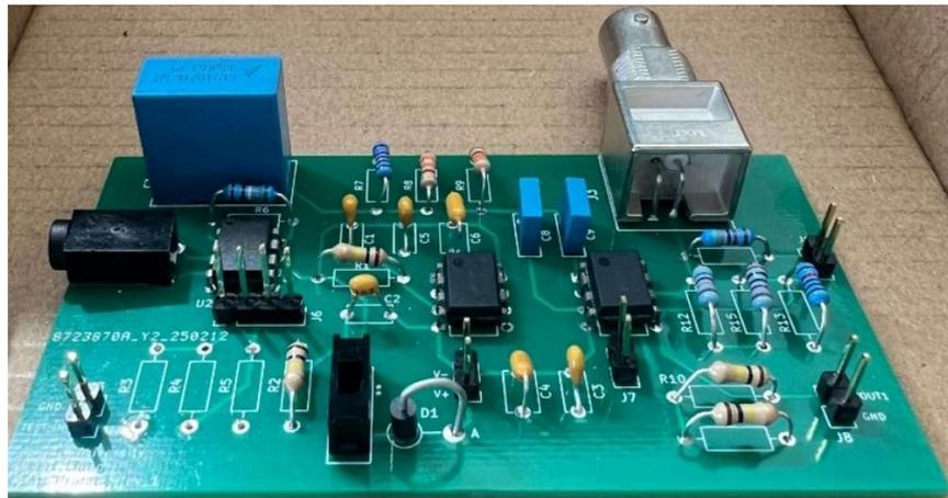
**Figure 14) Soldered PCB Assembly (Rev\_01)**
