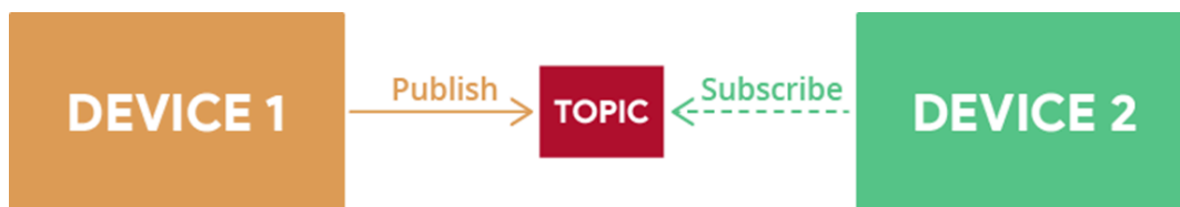
Figure 1: MQTT Communication System [5]
