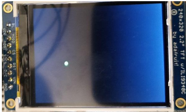
Fig. 23 Testing the TFT Library with bouncing ball code
