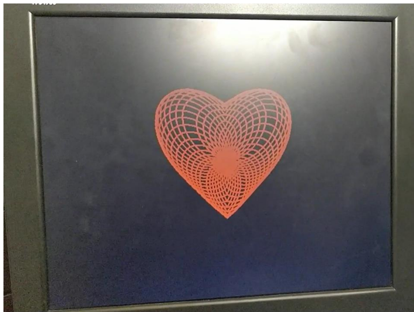
Fig. 20 Plotting the equation on a VGA screen using RaspberryPi Pico
