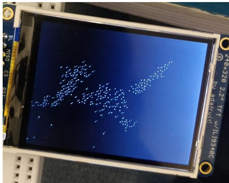
Fig. 24 Testing the TFT Library with boids algorithm
