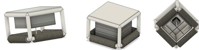
All components will be mounted into a floating chamber. There is a telescopic structure inside the chamber. When the telescopic structure drop down, it will touch the water surface and generate a sealed space in order to let sensor collect accuracy and unchanged data. After each measurement, the structure will go up and refresh the air inside the chamber, and be prepared for the next round of measurements.
