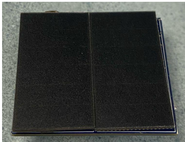
Figure 31: SolarTracker Board with solar cells mounted. Reverse side has all ICs as shown in Figure 28.
