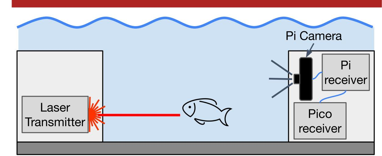
The reef consists of 2 waterproof enclosures mounted on an acrylic base.
