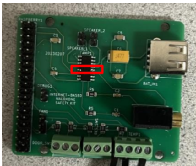
Figure 8: First Version PCB Prototype. The pins in the red rectangle were connected to the GND by mistake.
