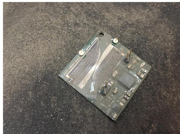
Fig. 6 Impact test article on bed of lunar regolith simulant after exposure to 27,000g of acceleration to simulate impact with the lunar surface.
