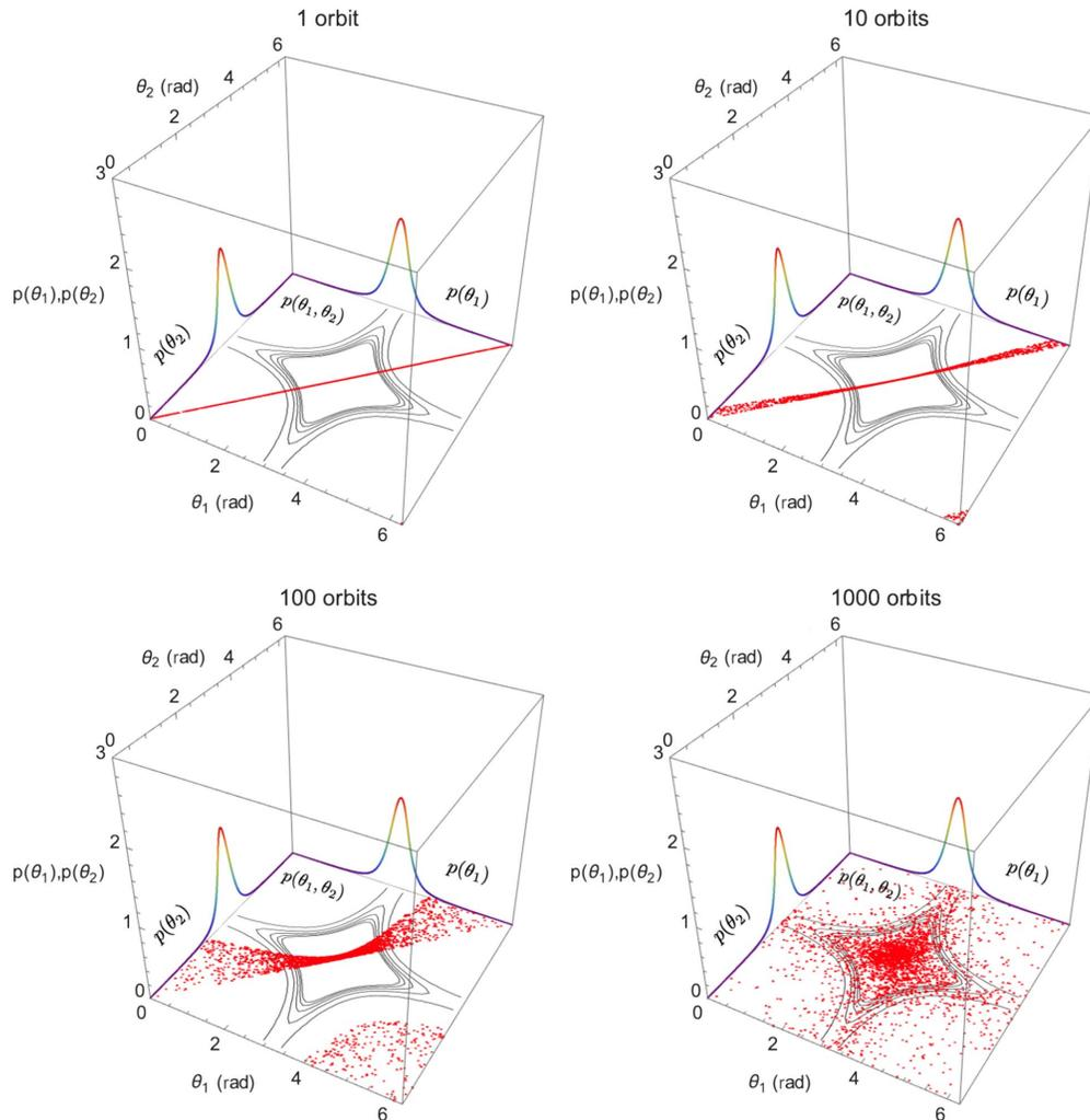
Fig. 5 True anomalies of two Monarchs deployed on orbits at geostationary altitude and inclination after varying numbers of orbits. Orbits are identical, except a variation in eccentricity by one-tenth of a percent.
