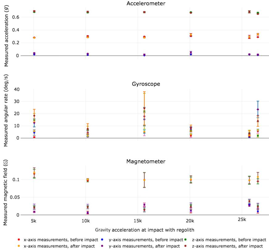
**Fig. 7** IMU measurements before and after impact with lunar regolith simulant, showing that the Microelectromechanical (MEM)’s sensor survives and continues to operate to within the specifications of the datasheet [36].
