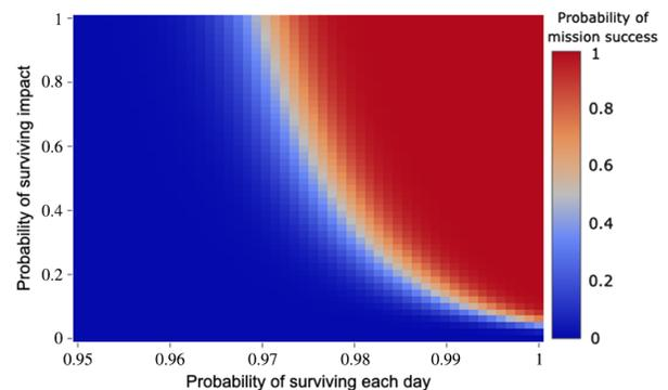
**Fig. 8** Probability of mission success, defined as 5 of 100 chipsats surviving on the surface of a celestial body for 100 days, for a range of impact survival probabilities and daily survival probabilities.
