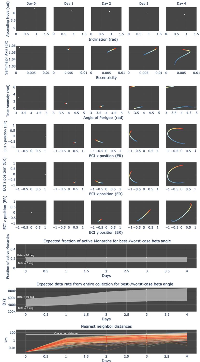
**Fig. 3** Five-hundred Monarchs deployed from International Space Station: plots of each Monarch’s orbital elements, Earth-centered inertial position, and distance to nearest neighbor (individually colorized); and plots of range of expected fraction of active Monarchs and expected range of data rates from collection.
