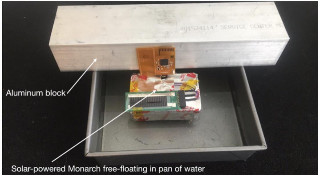
Figure 2.6: Test setup for torque coil actuation demo.
