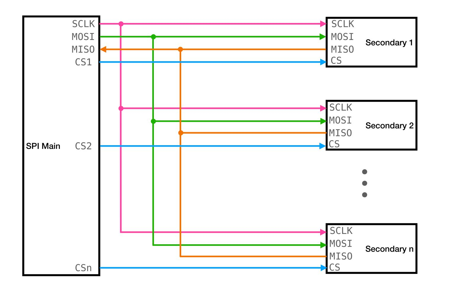
Different manufacturers often call these lines by different names. Read the datasheet! If you understand the function of each line in the SPI protocol, then you will understand which to connect, even if they have different naming conventions.
