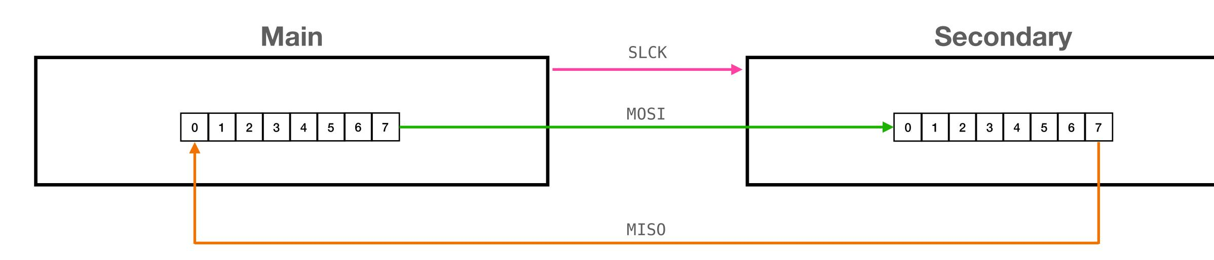
When the master loads the transmit register (int, short, or byte), the transmit begins. Data is simultaneously and synchronously sent from master to peripheral, and from peripheral to master over the MOSI/MISO lines.
