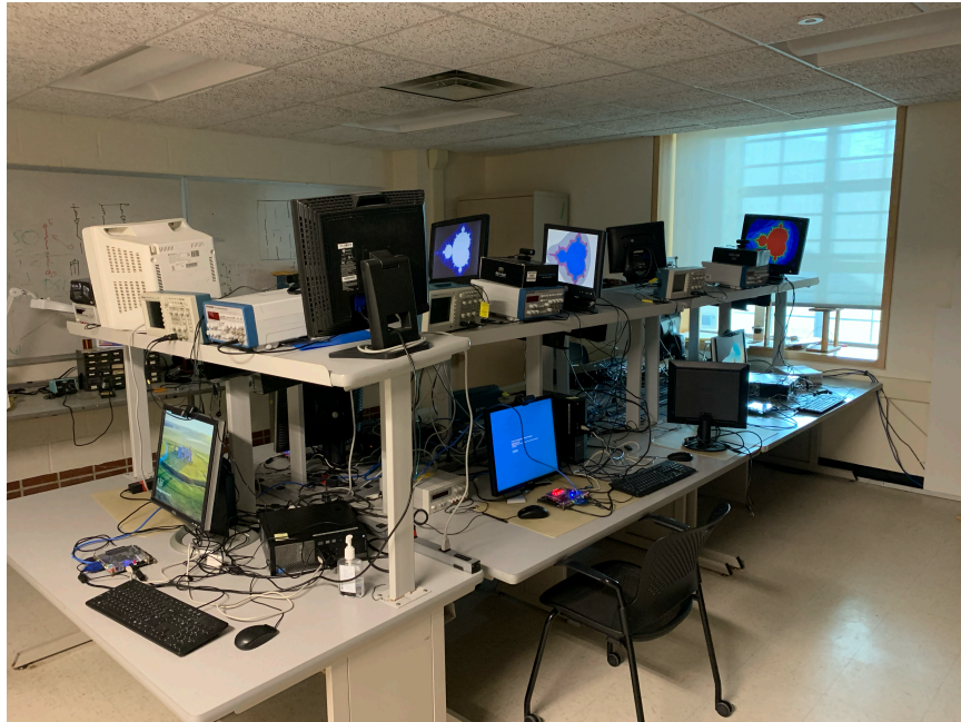
Fig. 1: Collection of remotely-accessible workstations for ECE 5760, Fall 2020. Each VGA screen shows a student in progress on the Mandelbrot lab assignment. Each workbench includes an FPGA and VGA, each observable via webcam, and an AUX cable from line out of the FPGA audio codec to the PC.
